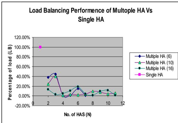
Fig.7. Comparison result for the (%) of load of each HA within 200s for single HA and multiple HA (N =6, 10, 16 & MN = 30).
