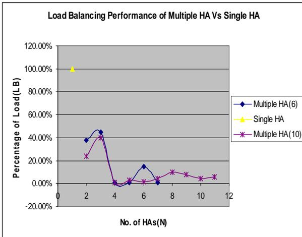
Fig. 6. Comparison result for the (%) of load of each HA within 200s for single HA and multiple HA (N =6, 10 & MN = 30).
