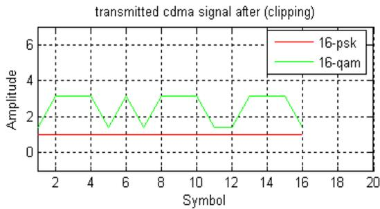
Fig.8 Transmitted CDMA signal after clipping.
