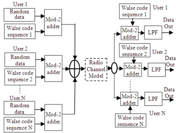
Fig. 3. CDMA model for multipath delay spread.
