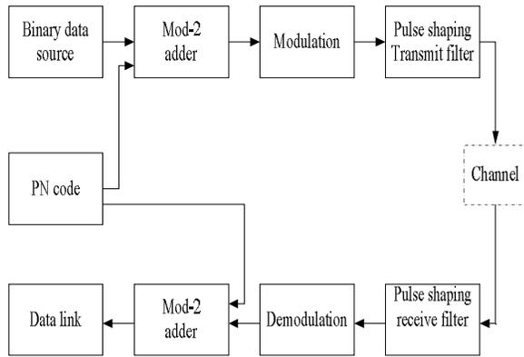
Fig. 5. Block diagram of CDMA model used for Doppler Effect.
