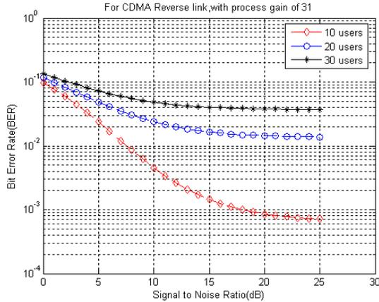
Fig. 2. BER vs. SNR of the radio channel for the reverse link of the CDMA system.
