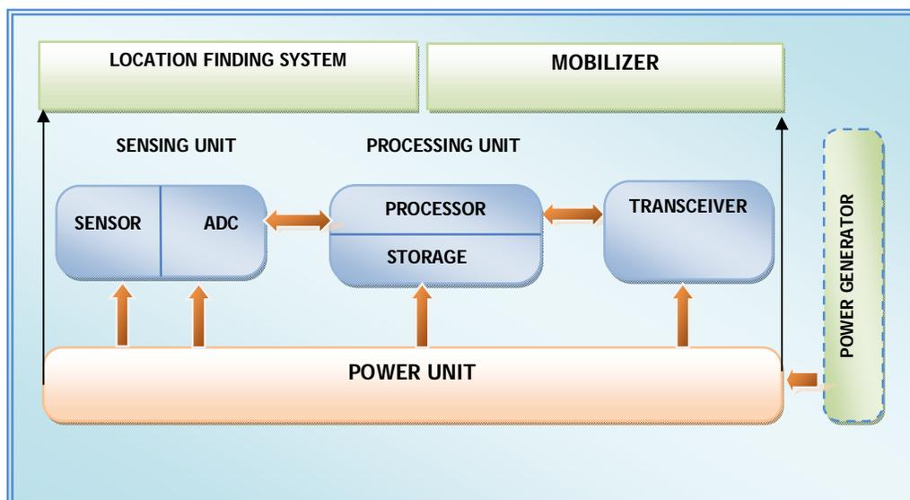
Fig. 2. Components of a Sensor Network
