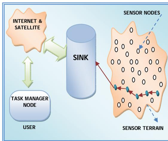
Fig. 1. Generic view of Sensor Network.
